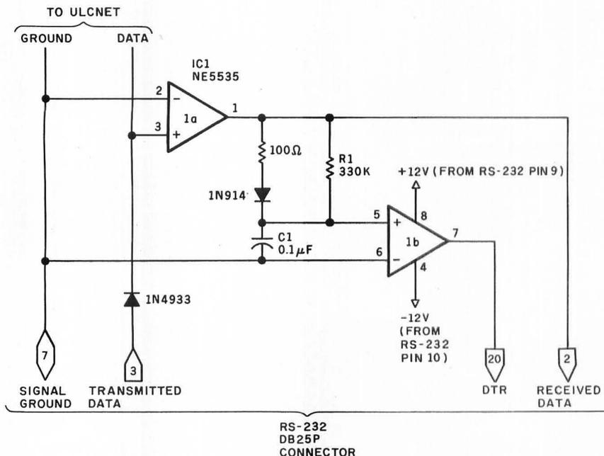
**Figure 3:** Simple modifications expand network capacity. An operational amplifier reduces the load placed on the net by each node, so that a virtually unlimited number of nodes can be used. Resistor R1 and capacitor C1 control the op-amp comparator to signal that the network is busy. The components shown can be used with speeds as low as 1200 bps; see table 1 for alternate selections.
